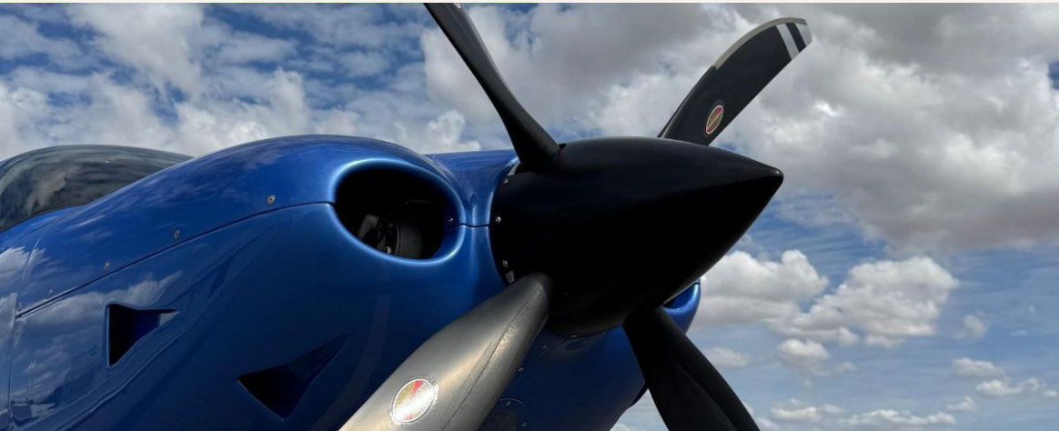
ENGINE INTAKE & FOUR BLADE COMPOSITE HARTZELL PROPELLER
